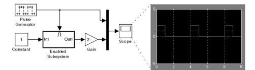
Simulink computes the outputs of the Constant block and Gain Block only when the Enabled Subsystem executes (i.e., at time steps 0, 4, 8, and so on). This is because the output of the Constant block is required and the input of the Gain block changes only when the Enabled Subsystem executes. When CE behavior is off, Simulink computes the outputs of the Constant and Gain blocks at every time step, regardless of whether the outputs are needed or change.
